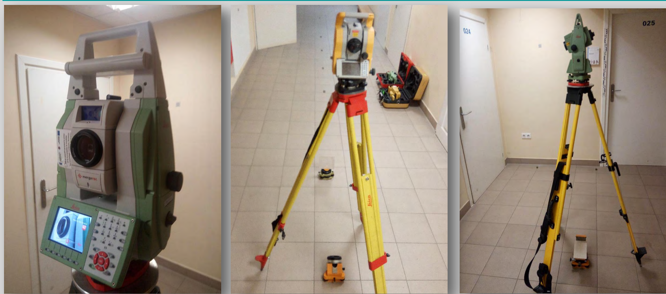
Figure 1 View of the tested instruments set up on classical tripod stands
